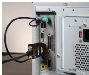
Direct connect CAT5 Transmitter streamlines your installation
